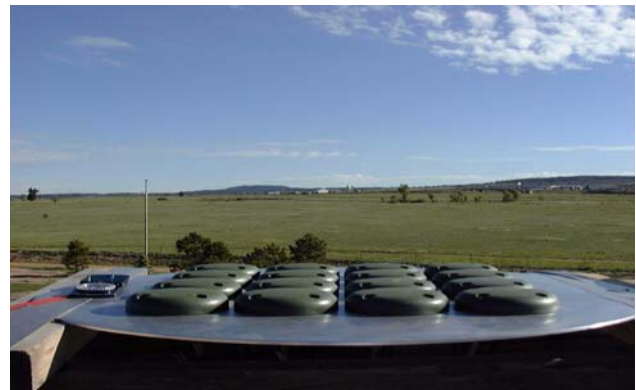
Figure 2 Sixteen Element L1/L2 Antenna Array
