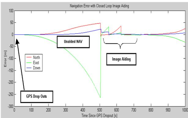
**Figure 10 Airborne Navigation with Image Aiding**
