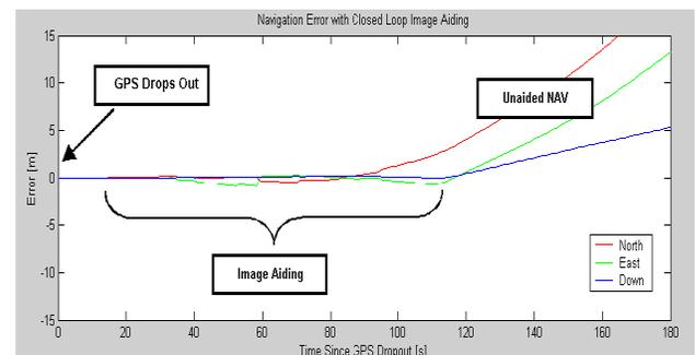
**Figure 12 Terrestrial Navigation with Image Aiding**
