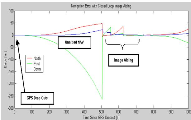
**Figure 10 Airborne Navigation with Image Aiding**
