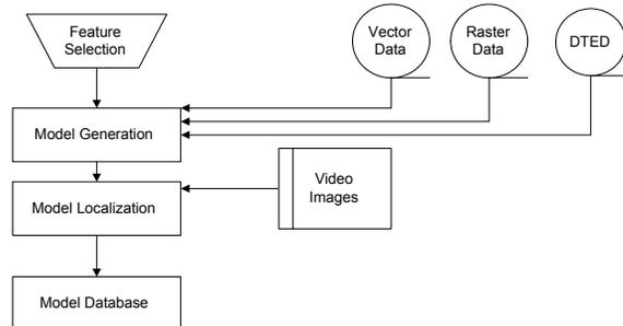
Figure 5 Model Generation Process
