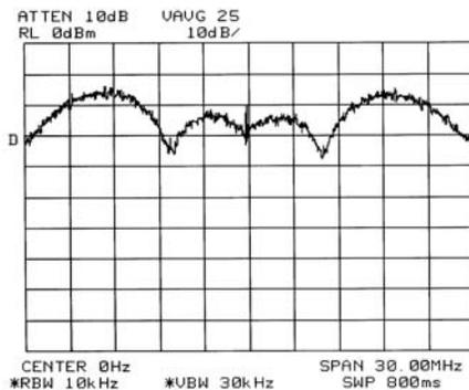
Figure 14 M-code modulation from CAC output
