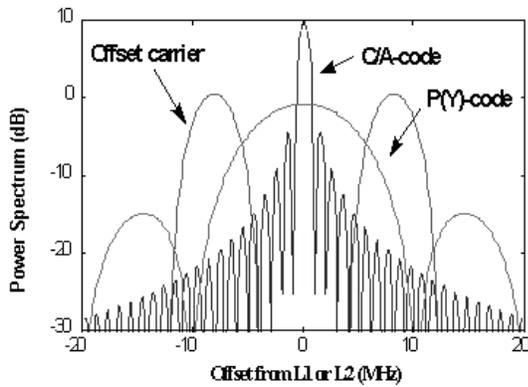
**Figure 1 C/A, P and M-code Spectral Characteristics**
