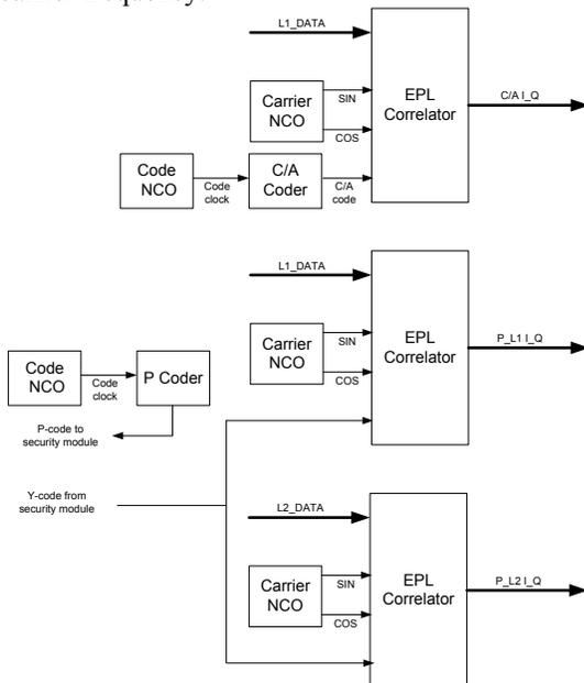
**Figure 8 CAC Channel Firmware Blocks**
