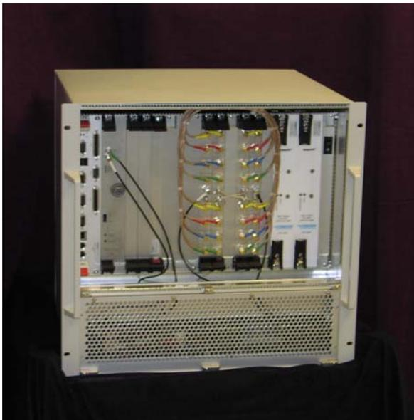
**Figure 5 SGR Test-Bed Rack Mounted Configuration Correlator Accelerator Card (CAC)**
