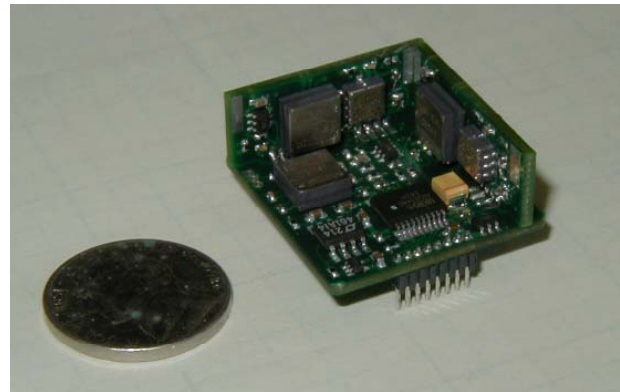
Figure 7 Small MEMS Inertial Measurement Unit (1"x1"x 0.5")
