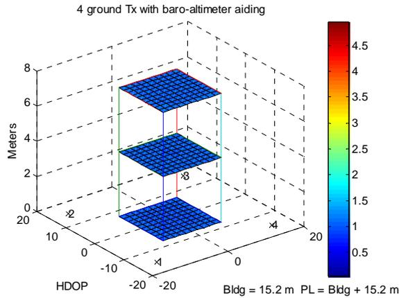
**Figure 7 HDOP with 4 Ground-based Transmitters and Altitude-aiding**
