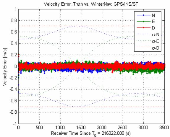
Figure 9 GPS/INS/ST Velocity Estimation Error
