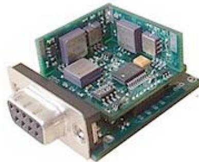
Figure 5 Cloud Cap Crista IMU
