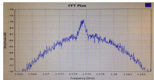
Figure 10 - Signal Spectrum without Interference
