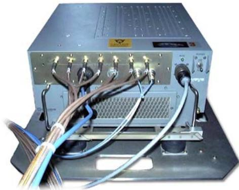
**Figure 6 HAGR-A Digital Beam Forming UTC GPS/Inertial Receiver**
