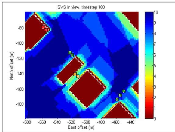
**Figure 3-3 Example Satellite Visibility View**
