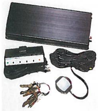
The in-vehicle unit's button-box driver interface can be attached to the driver's sun visor or kept in the glove compartment.
